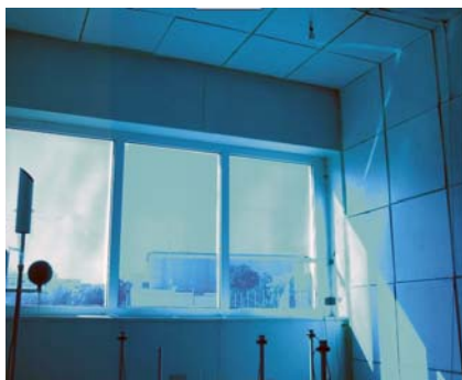
Figure 6 Picture of inside view of PASSYS cell at coloured EC-windows on 30.08.2005, 9.00 p.m.
