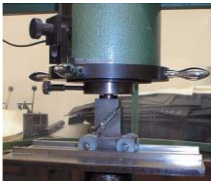
Figure 8: Compressive shear strength test apparatus
